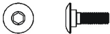
Socket button head collar screw 半圓頭內六角軸套螺絲(M3x10mm) x 2
