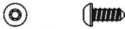
Socket button head self tapping screw 半圓頭內六角自攻螺絲(T2.6x6mm) x 1
